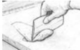
Applying an epoxy fillet to any external angles will allow the fabric to be easily laid.
