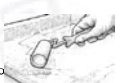
**NOTE:** If working on uncoated wooden surfaces, ensure the timber is warmed before application of epoxy. Remove the heat source before applying the epoxy. This will eliminate the "out-gassing" produced when expanding air is released from the wood fibres. If the surface is to be clear finished, use lighter weight fabrics, although one layer of 280 g/m<sup>2</sup> Twill fabric will become transparent, the weave of the cloth may still be visible.
