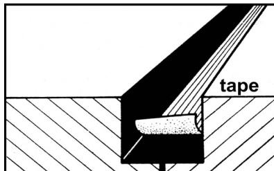
Apply separation tape at the bottom of the joint to avoid 3-side bonding.
