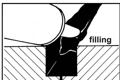
Fill the joints excessively with TDS Caulking from the bottom up to avoid locking in air bubbles. Use a spatula to slightly smoothen the sealant without applying any pressure.
