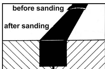
After curing: cut away excess material using 80 grit paper and then sand the deck using an oscillating sanding machine
